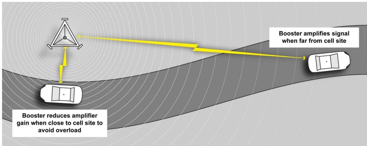
As you approach the cell site, less and less boost of your phone's signal is required. In this situation, the amplifier reduces the gain, or if necessary, shuts off completely. Thus at no time is the cell site overloaded with too strong a signal. Then, as you move away from the site and signal amplification is required, the booster comes back on (if it shut down) and continually varies its gain for optimal performance.
