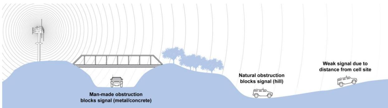
Poor signal strength has another effect on your phone's performance. Wireless networks are designed to minimize the amount of power necessary for your phone to communicate with the cell site. The closer you are to a site, the less power required from your phone and the longer your battery life. Conversely, the further you are from a cell site, or the more obstacles between your phone and the cell site, the more power the phone must use to communicate, and this will shorten its battery life
